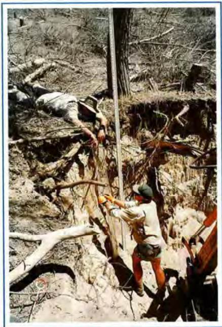
4b. Image showing researchers measuring the roots of a stressed cottonwood on Mojave River with depth to groundwater exceeding plant requirements. Source: Lines 1999.
