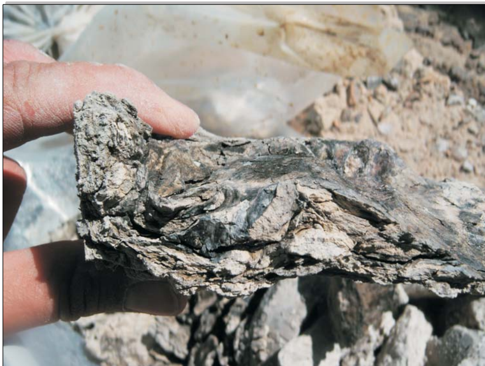
Cluster D - partially lithified, foliated clay, 192.5' - 195'
