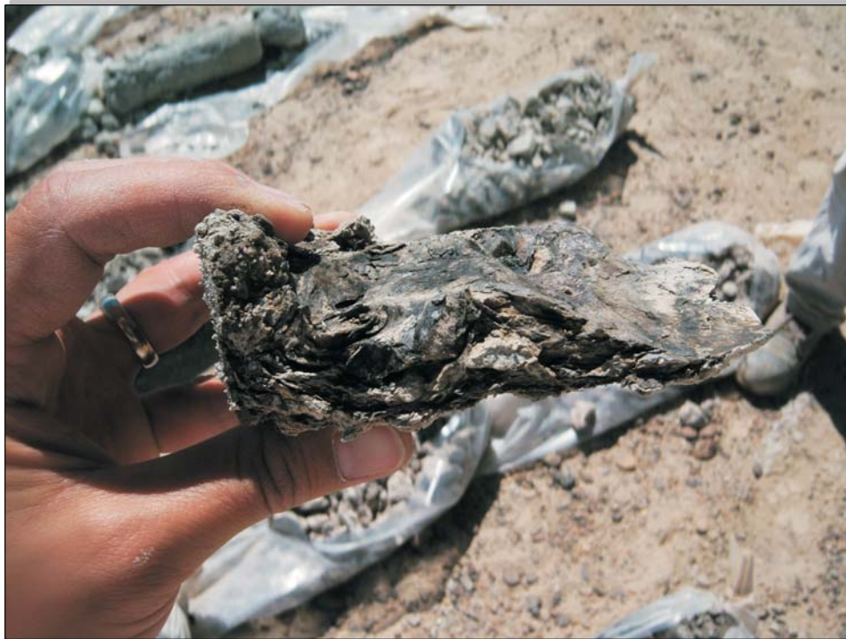
Cluster D - partially lithified, foliated clay, 185' - 187.5'
