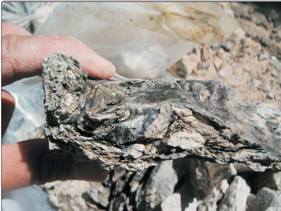
Cluster D - partially lithified, foliated clay, 192.5' - 195'
