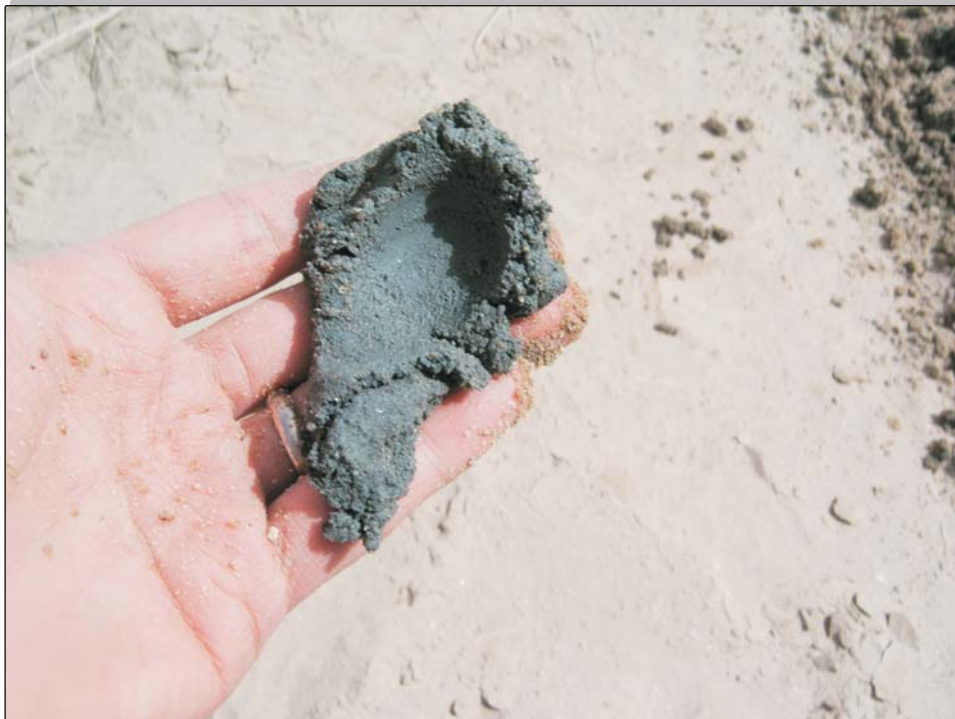
Silt/Clay encountered at bottom of Shallow Piezometer P8
