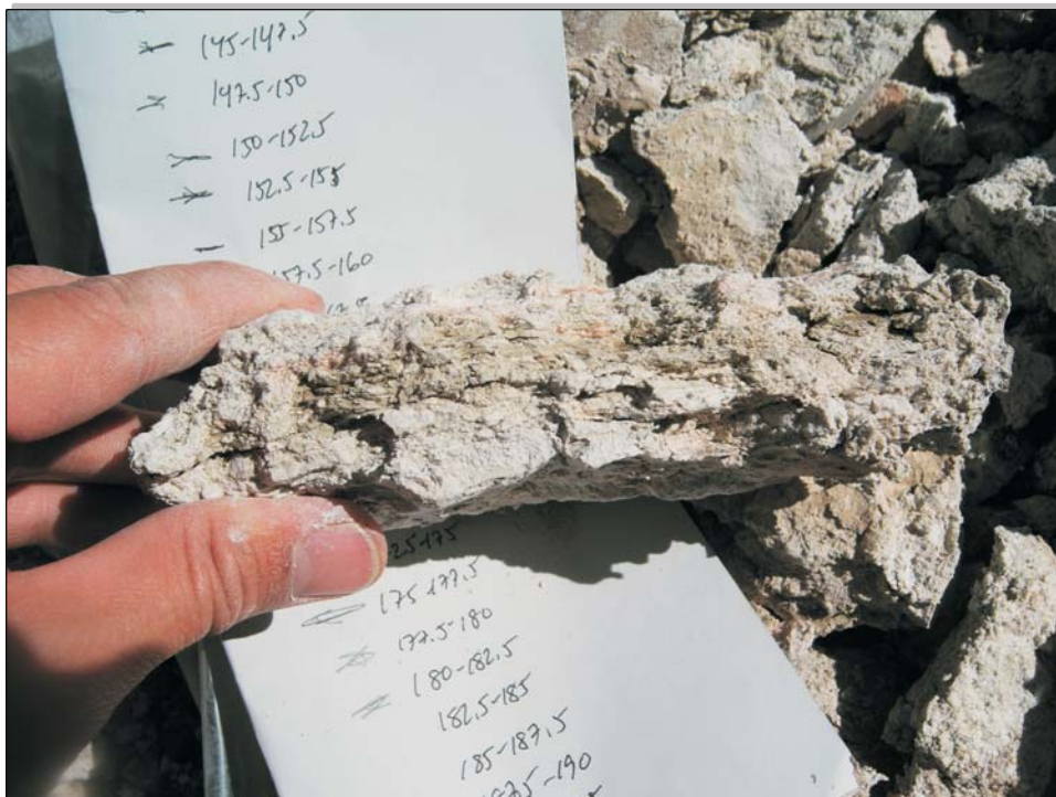
Cluster D - cemented, friable, partially lithified silt/clay, 180' - 182.5'
