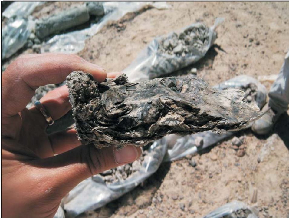
Cluster D - partially lithified, foliated clay, 185' - 187.5'
