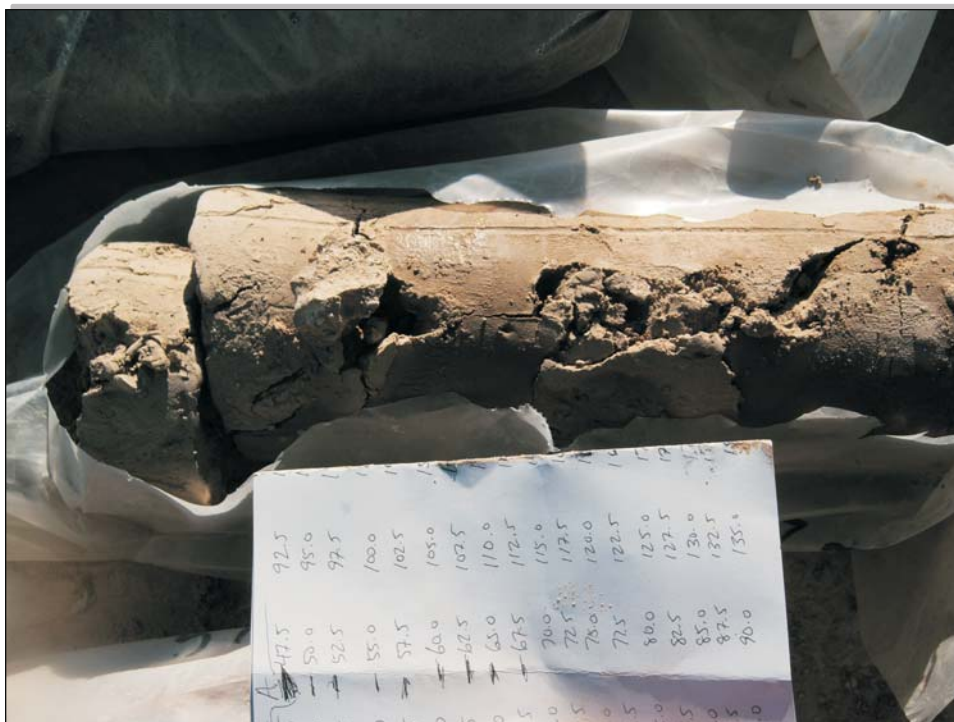
Cluster A - Manix Clay Beds (oxidized), 65' - 67.5'
