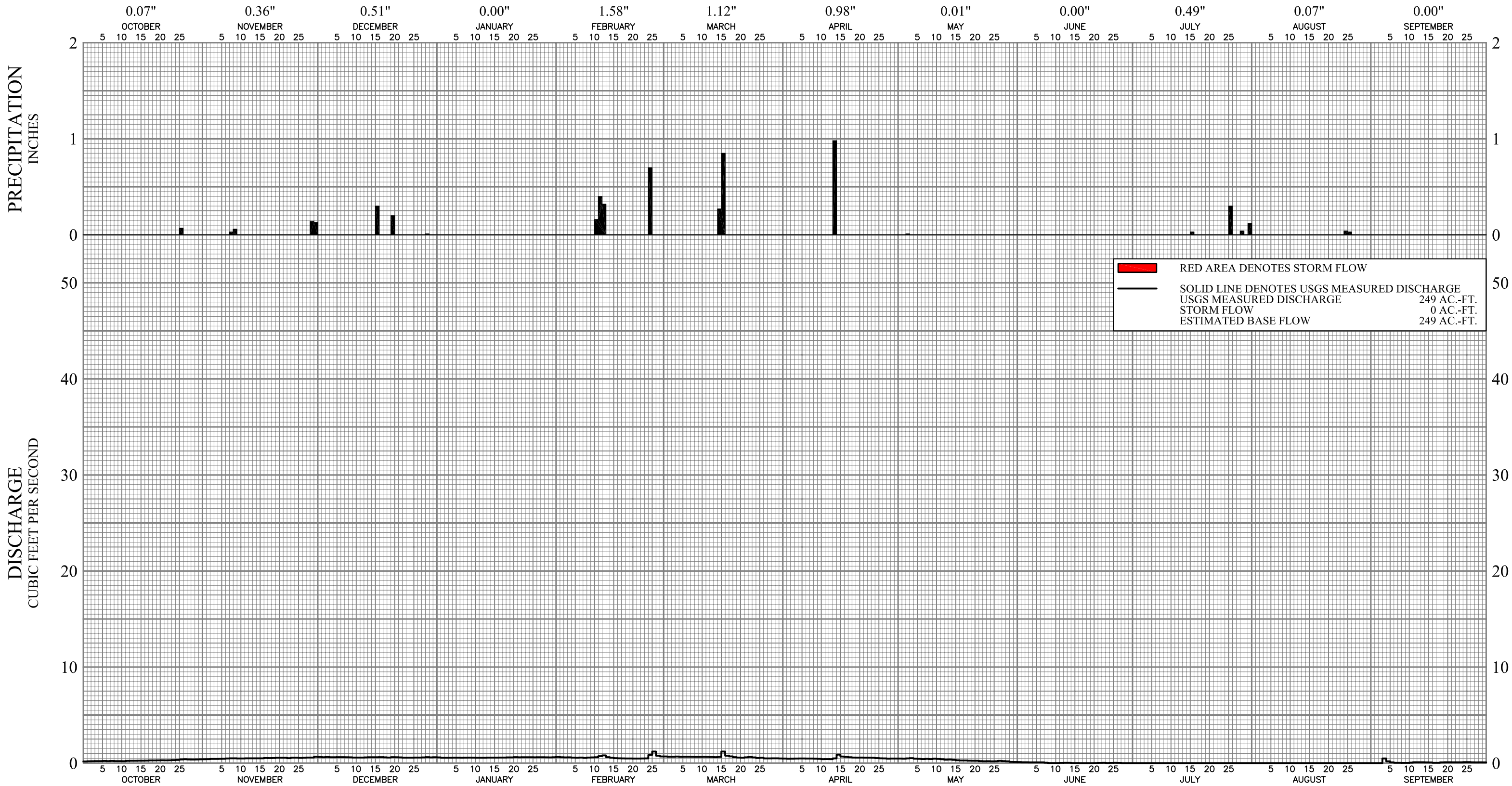
DISCHARGE OF MOJAVE RIVER AT AFTON AND PRECIPITATION AT BARSTOW WATER YEAR 2002-03
